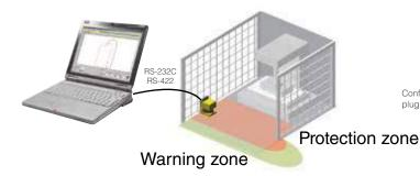
Monitors beam misalignment after installation of safety laser scanner
