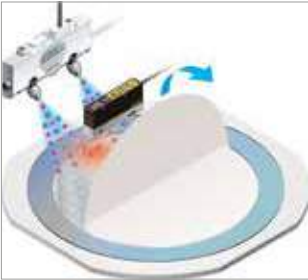
Measuring surface potential when removing BG sheets
