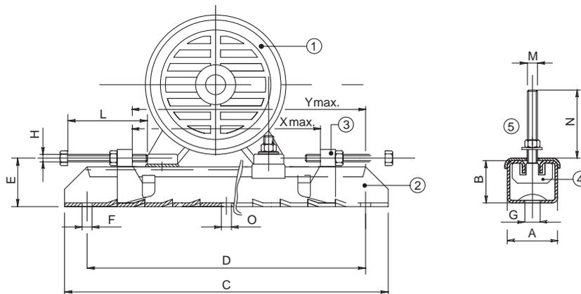
1 Motor | 2 Rail | 3 Movable adjusting bolt | 4 Fixing bolt, motor | 5 Plate
