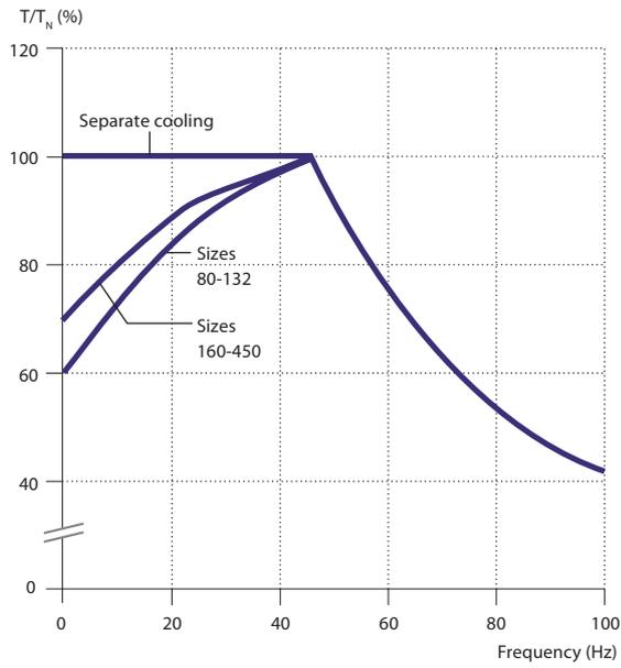
Figure 2a. Loadability curves for frequency converters with DTC control
