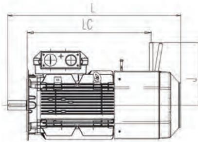
Flange-mounted: IM B5 (IM 3001), IM V1 (IM 3011), IM V3 (IM 3031), IM B14 (IM 3601), IM V18 (IM 3611), IM V19 (IM 3631)
