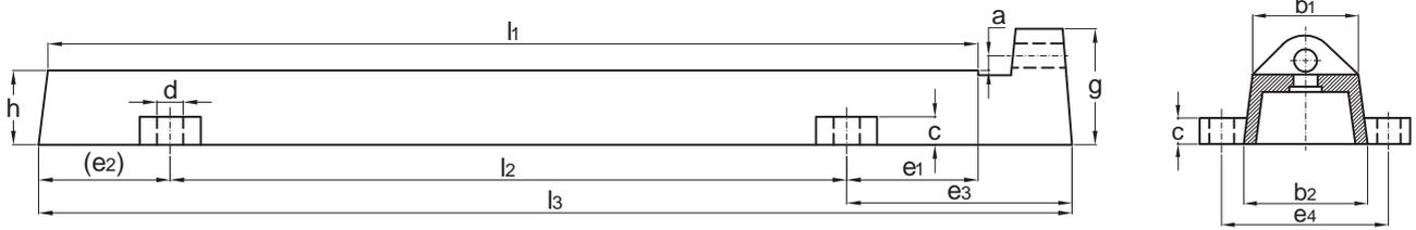
Slide rails for motor sizes 280 - 315.
