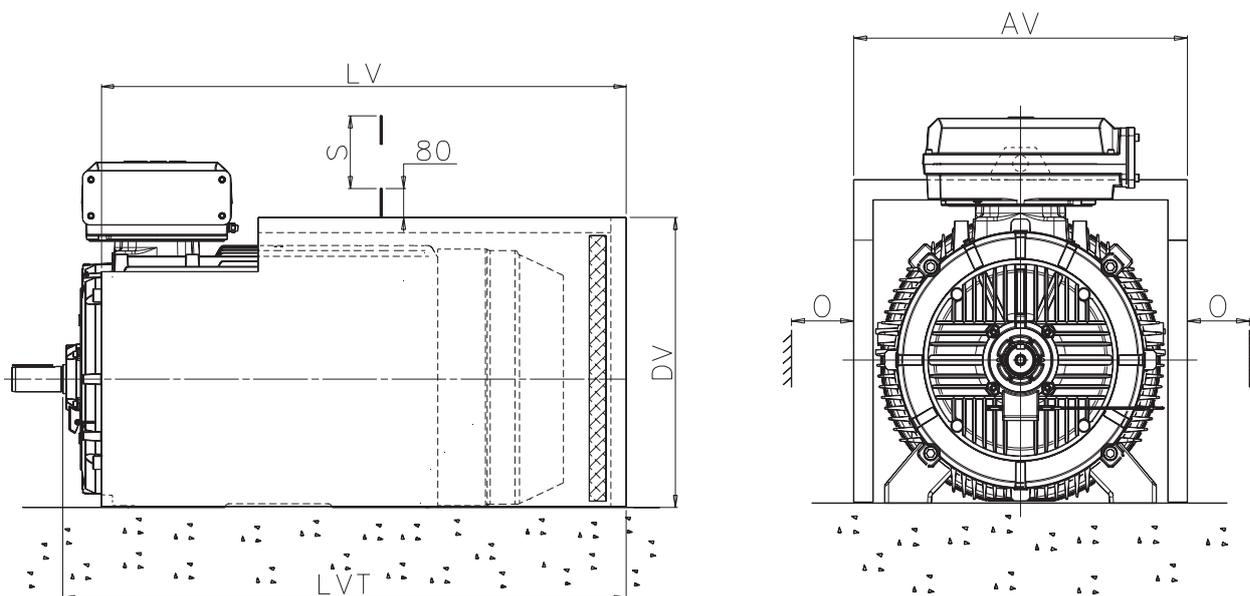
Both foot-mounted and flange-mounted motors can be fitted with a silencer to reduce noise level by about 5 - 6 dB(A). The silencer is painted blue and made of 2 mm steel sheet. The sound absorbing material is 40 mm thick polyurethane foam. On the rim there is a rubber strip for sealing on the floor. The silencer fits loosely over the motor.
