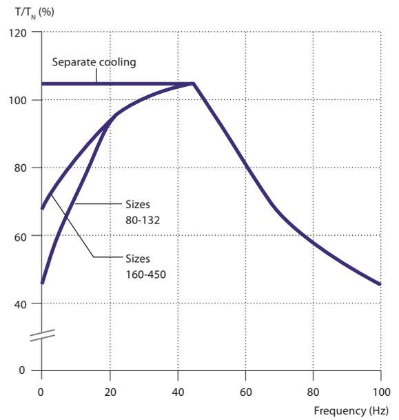
Figure 3b. Loadability curves for other frequency converters
