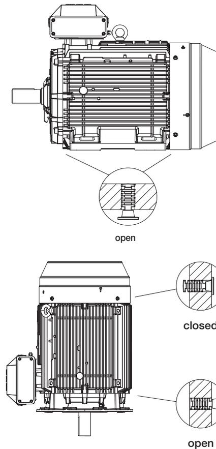
As standard, motor sizes 71 - 450 are delivered with drain holes and closable plugs.
