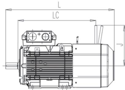
Foot-mounted: IM B3 (IM1001), IM B6 (IM 1051), IM B7 (IM1061), IM B8 (IM 1071), IM V5 (IM 1011), IM V6 (IM 1031)
