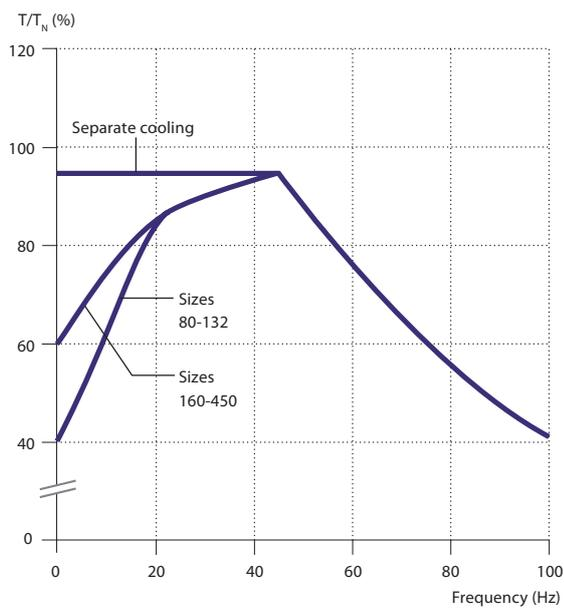
Figure 2b. Loadability curves for other frequency converters
